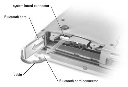
**NOTE:** When replacing the Bluetooth card, ensure the Bluetooth cable is routed correctly so that you do not damage the cable when you install the hard drive.
